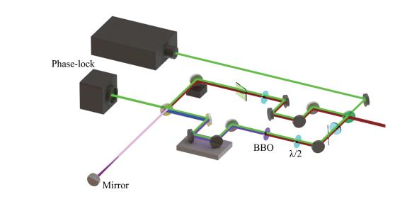
FIG. S1: Schematic view of phase-locked Mach-Zehnder interferometer scheme.
